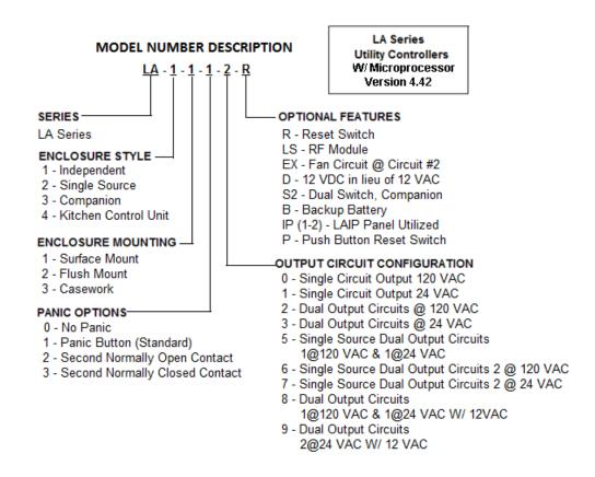
NOTE: Output Configurations 5, 6, 7, 8 and 9 are intended to operate with specific operators and solenoids for applications such as Instructor's Demonstration Stations and 8 cience Preparation Rooms. When Configurations 2 or 3 are specified with Single Source Units, then Outputs are typically provided as single switch operators with or without a Reset per each output.
